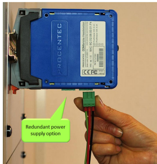
Powering the Head Station
